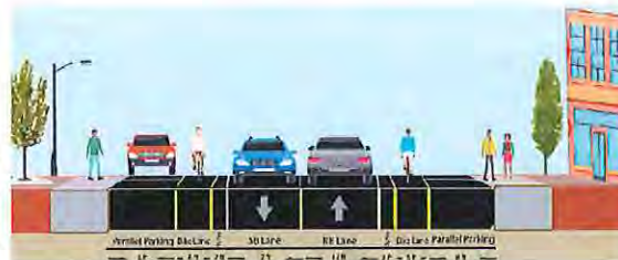
Alternative Two-Way Typical Sections with Left Turn Lane (top) and bicycle lanes (bottom)
